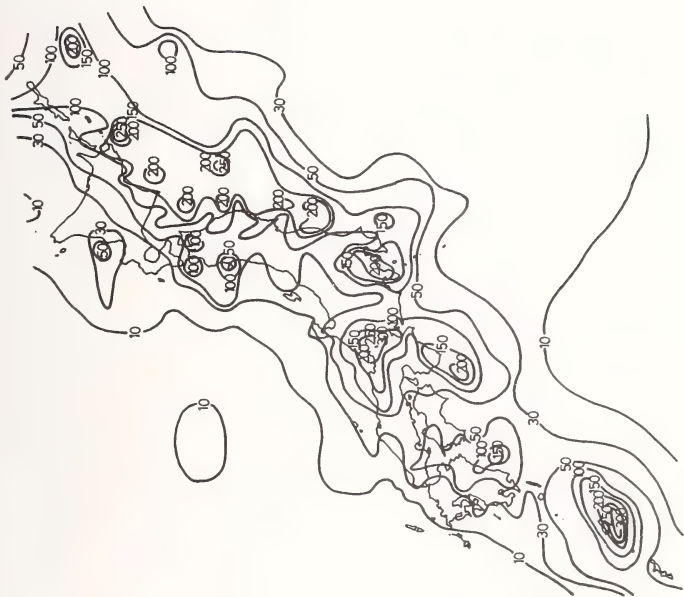
Fig. 15. Regional Distribution of the Expected Displacement Values (cm) at the Base Rock ( T_G=5.0 sec., t=100 years)
